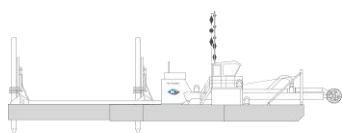
Nu Compact Cutter Suction Dredge
